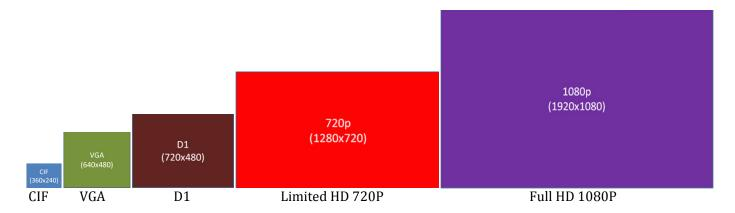
CIF About useless due to the low-resolution, poor images, currently used in low bandwidth video streaming.
