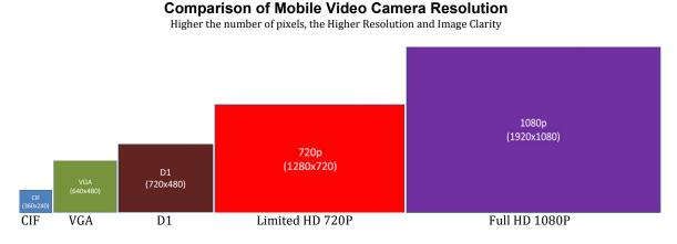
CIF About useless due to the low-resolution, poor images, currently used in low bandwidth video streaming.
