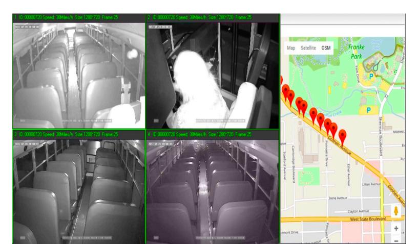
SD4HW Night Vision IR LEDs active for recording in total darkness, OSM map setting GPS breadcrumbs showing route SD4HW High Definition Road Facing camera, with IR LEDs disabled to prevent "ghosting" glare off windshield
