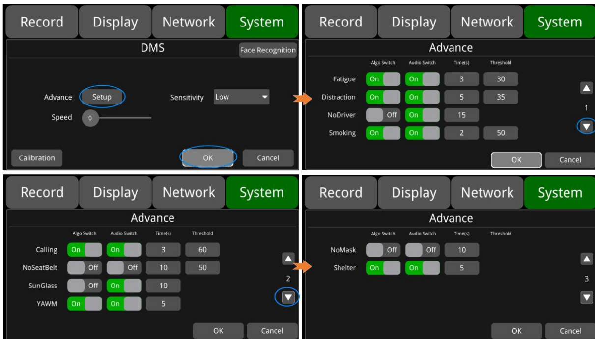
Algo switch Setup : DMS detection alarm type selection and default configuration.
