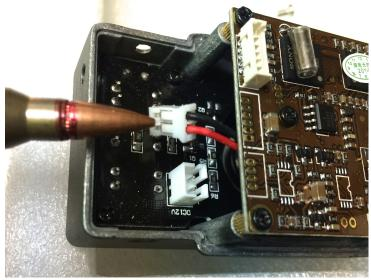
Cut the power wires and then insulate the power wires for safety considerations.
