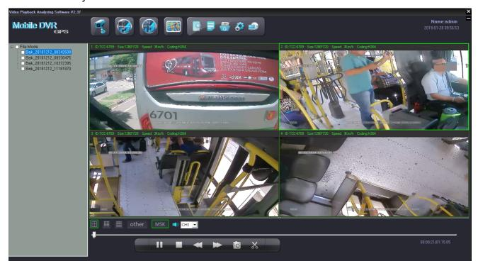
On the left side of the software, SD records info will be showed: UnlockFile and Lockfile will be displayed on the interface.
