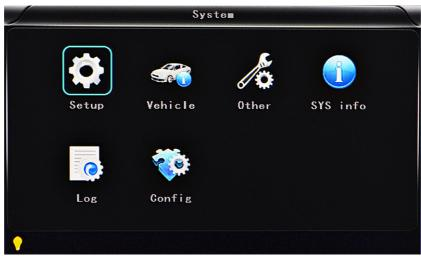
• Setup setting: includes options of "Base", "User", "Serial", "PTZ", "GPS", "G-sensor" and "NTP"
