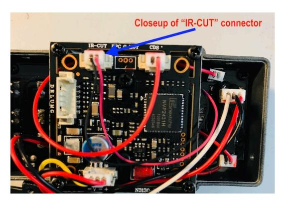
**4.How to disable the IR LED Power array board connector:** Unplug the connector in the below image to disable the IR LEDs.
