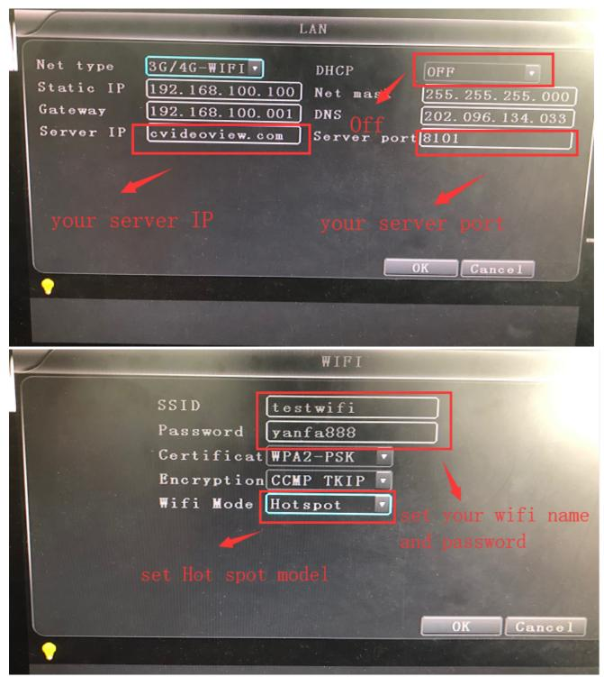
\*In the 3g/4g-wifi net type, set DHCP off, set to Hot spot mode, use 3g/4g to share flow to the user.at that time ,the SSID and Password is your WIFI name and connect password.
