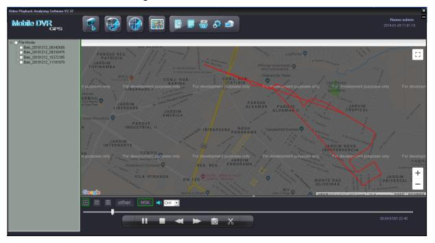
Open HDD :: used to search the hard disk connected with the computer and it will play the earliest recorded video after searching. (This button releases the limitation of the sequence- connecting hard disk or SD card to computers before opening the software and no need to close the software even connecting a new hard disk or sd card with recorded video). Open File Used to search the videos in computers or U-Disk or hard disk.
