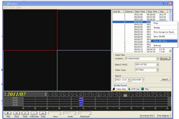
The GPS data extraction is now functional and it can extract the data into a "KML" file type that could be used by a mapping program to plot route location information on their maps. What would be required is to find a mapping program that can import the "KML" data into their map to create a route of that vehicle for that day.
