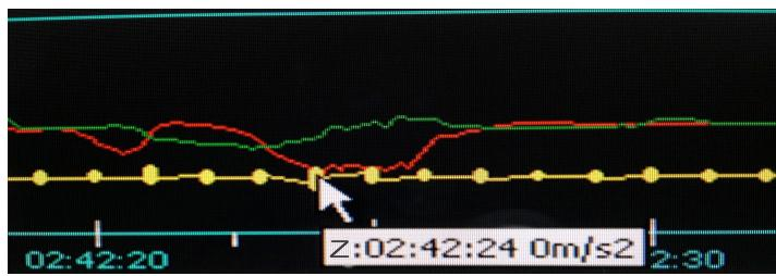
"Z" axis deflections can indicate sudden changes in up or down inertia, that can be caused by hitting large potholes, running over curbs or running over speed bumps at a high rate of speed. Anything that will cause the vehicle to drop down or bounce up will be reflected on the "Z" axis charting.
