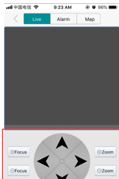
set for PTZ, you can adjust direction, lens focal length, zoom in and zoom out
