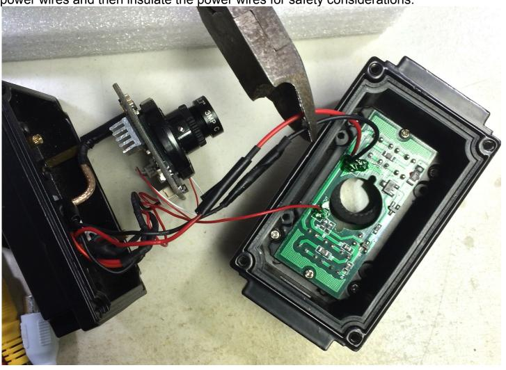
Step 5 Reassembly is the reverse of the above. Make sure you do not pinch any power wires.
